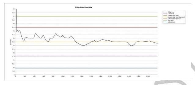
Ridge profile between Lake Srebarna and the Danube. At present, the connection between the Danube and Srebarna is through the stretch from 0 m to 800 m (a stretch of breached dike), theoretically at levels above 13.50 m a.s.l. (in practice at levels above 14.00 m a.s.l.).
